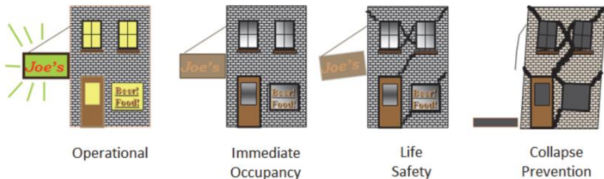
Figure 2. Standard ASCE/SEI 41 performance levels.
